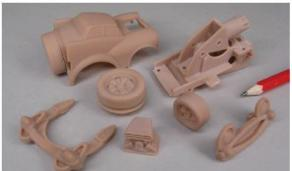
Yellow resin are high-temperature resins for building tough and stiff parts at very high resolutions. Parts made with these materials are ideal for silicone molding, pump housings, blades, test parts for wind tunnels, light reflectors and various automotive applications. These materials are also perfect for high detail jewelry and animation applications and can be finished with a variety of methods including painting or plating.
